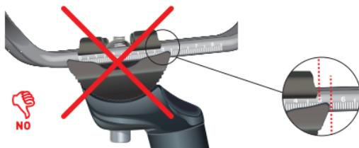
7. the jaws should not cause deformation or damage to the saddle frame
